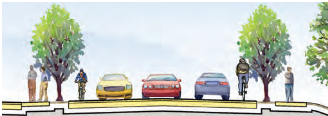
existing (above) and proposed (below) sections of Corrigan Drive showing lane reduction and added walks and bike lanes
